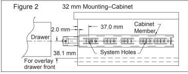
Use only the 32 mm system holes or the wood screw holes located at the tip of the breathing tabs. Do not use any other holes on the cabinet member for mounting (Figure 3).
