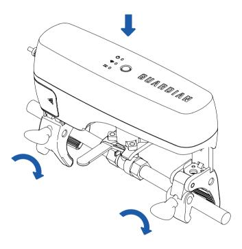
Hand Tighten Only - Do not use tools to tighten/adjust clamps
