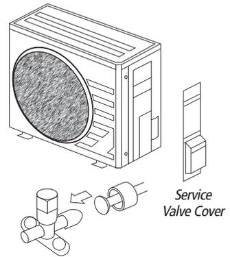
**NOTE:** Use proper techniques to cut and re-flare refrigerant pipes, if required. An R410A Flaring Tool is required for re-flaring refrigerant pipes.
