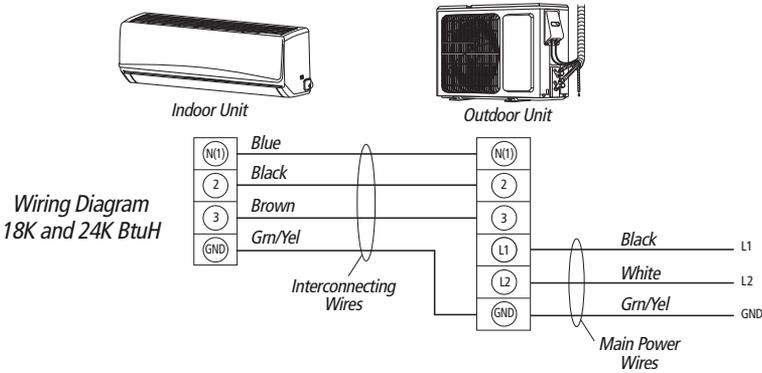
5. Following the same wire colors and terminal references from the indoor unit, tightly connect interconnecting wires to the outdoor unit terminal block per wiring diagram above.
