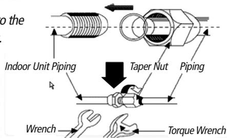
10. Carefully tighten flare nuts to correct torque level referring to the following Torque Table:
