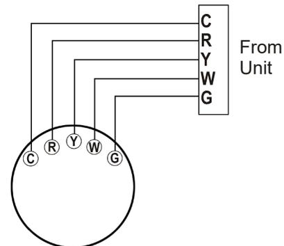
**SINGLE STAGE HEATING & COOLING THERMOSTAT DIAGRAM**
