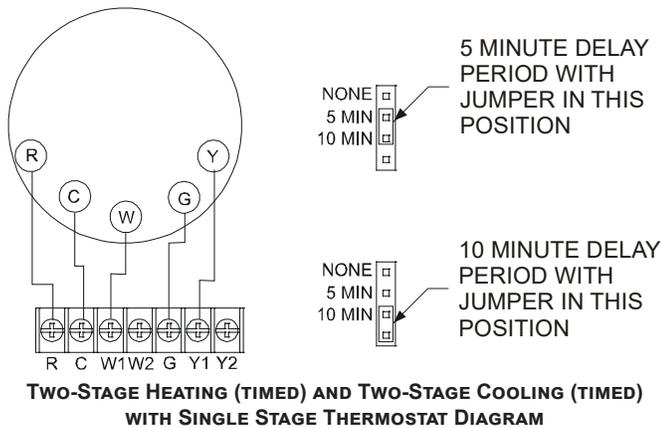
Refer to the unit wiring diagram for electrical connections. When installed, the unit must be electrically grounded in accordance with local codes or in the absence of local codes, with the National Electrical Code, ANSI/NFPA No. 70, and/or the CSA C22.1 Electrical Code. Ensure low voltage connections are waterproof.
