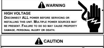
IF YOU MUST HANDLE THE ITNITOR, HANDLE WITH CARE. TOUCHING THE IGNITOR BODY WITH BARE FINGERS, ROUGH HANDLING, OR VIBRATION COULD RESULT IN EARLY IGNITOR FAILURE. ONLY A QUALIFIED SERVICER SHOULD EVER HANDLE THE IGNITOR.
