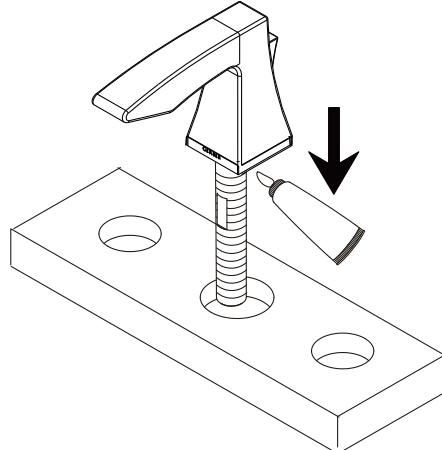
3. From underneath the sink, install the rubber washer, metal washer and lock nut. Thread on the adapter to the bottom of the spout shank, and tighten.
