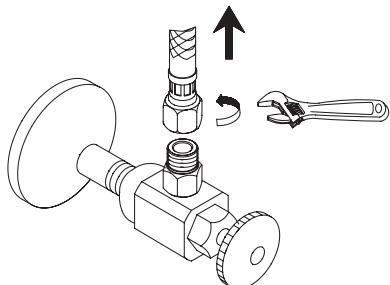
1. Remove the hose end from the the adapter using the adjustable wrench.
