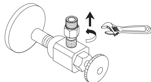
2. Remove the adapter from the water supply by using the adjustable wrench.
