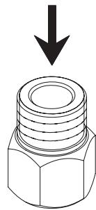
3. Flush out the debris on the restrictor inside the adapter.
