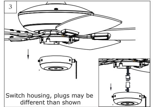
Unplug (If wiring with quick connectors) and remove the switch housing from fan.
