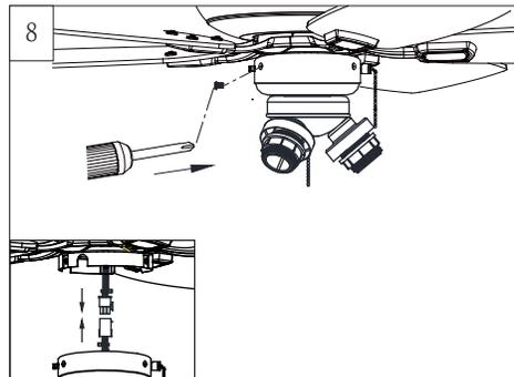
If wiring with plugs, connect the plug from fan to the plug from light kit assembly. Make sure the plugs are clasped firmly. Install light kit assembly (switch housing) onto the fan with the set screws removed in step 2.
