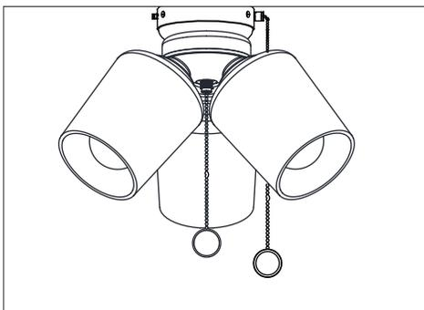
Install 3 x 9-watt medium base enclosed type of LED lamps.
