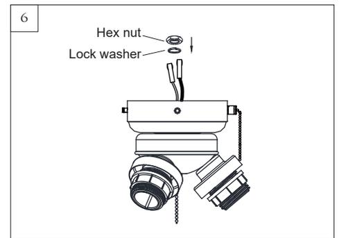
Place the lock washer and hex nut over lead wires from light fixture and tighten securely with the thread rod of light fixture.
