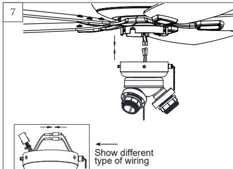
Connect white wire from light fixture with white wire from fan and then connect black (or blue) wire from light fixture with blue (or black) wire from fan.
