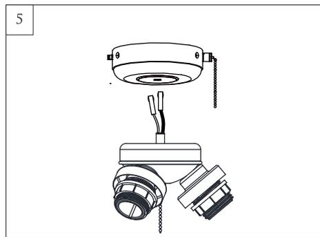
Thread lead wires from light fixture through central hole in switch housing and then install switch housing onto the light fixture by turning clockwise till tight.
