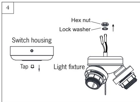
Remove tap from bottom of switch housing. Remove the hex nut and lock washer from the light fixture. Keep the hex nut and lock washer.
