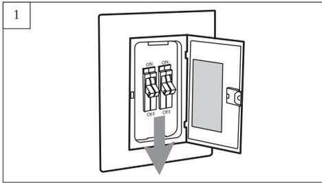
Before you begin installing the fan, Switch power off at Service panel and lock service disconnecting means to prevent power from being switched on accidentally. When the service disconnecting means cannot be locked, securely fasten a warning device, such as a tag, to the service panel.
