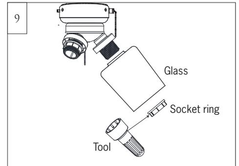
Screw out the socket ring, then push in the glass and lock in the socket ring by the tool provided.
