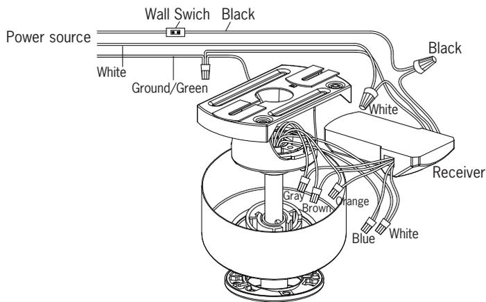
**Note:** For better performance of the remote operation, keep the WiFi antenna apart from the antenna of the receiver.
