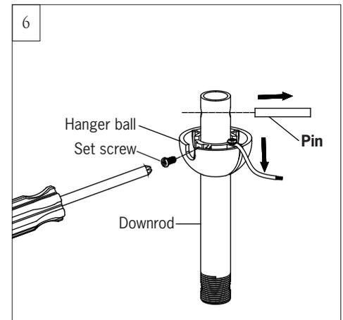
Remove hanger ball from downrod by loosening the set screw and removing the pin as shown in illustration. Keep parts.
