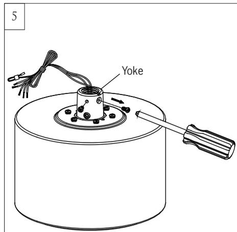
Remove downrod set screws from the yoke on top of motor assembly. Keep the screws.
