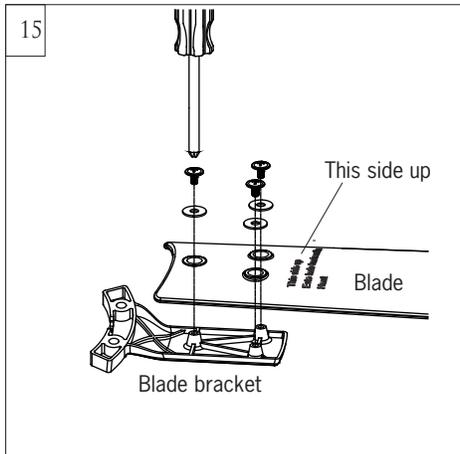
Install blade onto blade bracket with provided set screws and washers. Tighten screws securely. Repeat this process for remaining blades.
