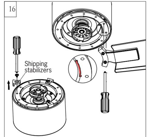
Remove shipping stabilizers from motor assembly.
