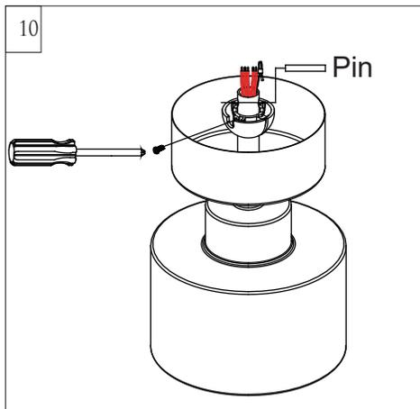
Replace the hanger ball with pin and set screw. Tighten it securely.
