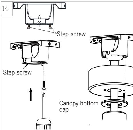
Partially loosen one and remove one preassembled step screw from mounting bracket (Do not remove the other set screws). Save the screw.
