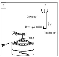
Partially loosen downrod set screws from yoke at top of motor assembly. Remove preassembled keeper pin and cross pin from downrod. Keep parts
