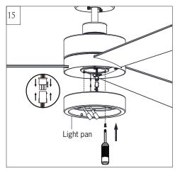
Connect the quick connector to the connector from the light pan. Be sure plugs connection clasped together firmly. Attach light pan onto the plate on motor, Place light pan over the lead wires from fan, aligning the keyhole slots on the light pan with the preassembled screws on the plate. Twist clockwise till lock. Reinstall the other screw. Tighten all screws securely.
