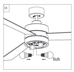
Install 2 x 9-watt medium base enclosed type of LED lamps.
