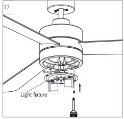
Connect white wire from fan to white wire from light fixture and then connect blue (or black) wire from fan to black (or blue) wire from light fixture. Be sure plugs connection clasped together firmly. Attach light fixture onto the light pan, aligning the keyhole slots on the light fixture with the preassembled screws on the light pan. Twist clockwise till lock. Reinstall the other screw. Tighten all screws securely.
