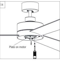
Loosen 2 and remove 1 preassembled screw from the plate on motor. Save screw for later use.
