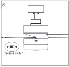
Setting the reverse switch on the left hand side will result in downward airflow and setting the switch on the right hand side will result in upward airflow.
