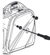
Figure 4-3. Remove Side Cover
