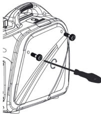
Figure 2-6. Remove Side Cover
