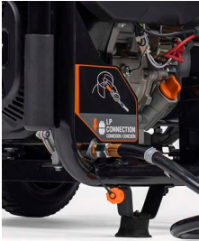
Figure 2-15. Connect Hose to Regulator
