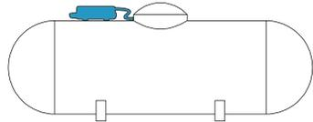
On **horizontal tanks**, mount the monitor on top of the tank.
