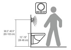
Installing highly reflective surfaces (such as mirrors) in the immediate vicinity of the water closet flush control should be avoided, as these can lead to incorrect releases and malfunctions.
