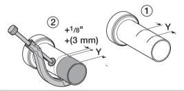
Bevel the sharp edges as shown to assure a smooth insertion into the pipe hubs in the wall.
