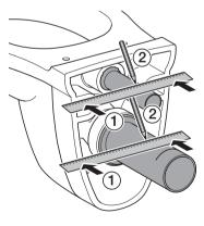
Add dimension X and 1/8". Using that dimension, mark a line on the pipe measuring from the hub side. Cut off the pipe at the line with a pipe cutter.
