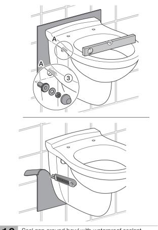
10 Seal gap around bowl with waterproof sealant.
