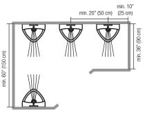
With urinal flush controls a minimum distance of 36" (90 cm) to the opposite wall must be observed to ensure problem-free detection. If urinal flush controls are mounted on opposite walls, a distance of 60" (150 cm) must be observed. Urinal flush controls mounted next to one another must be at least 20" (50 cm) apart.
