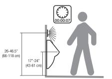
Installing highly reflective surfaces (such as mirrors) in the immediate vicinity of the urinal flush control should be avoided, as these can lead to incorrect releases and malfunctions. Geberit product is ADA compliant when fixture and actuator are installed at proper heights.
