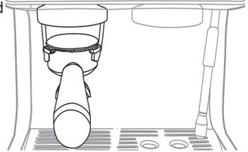
5. When grinding is complete, remove the portafilter and gently tap to even out the coffee grounds.
