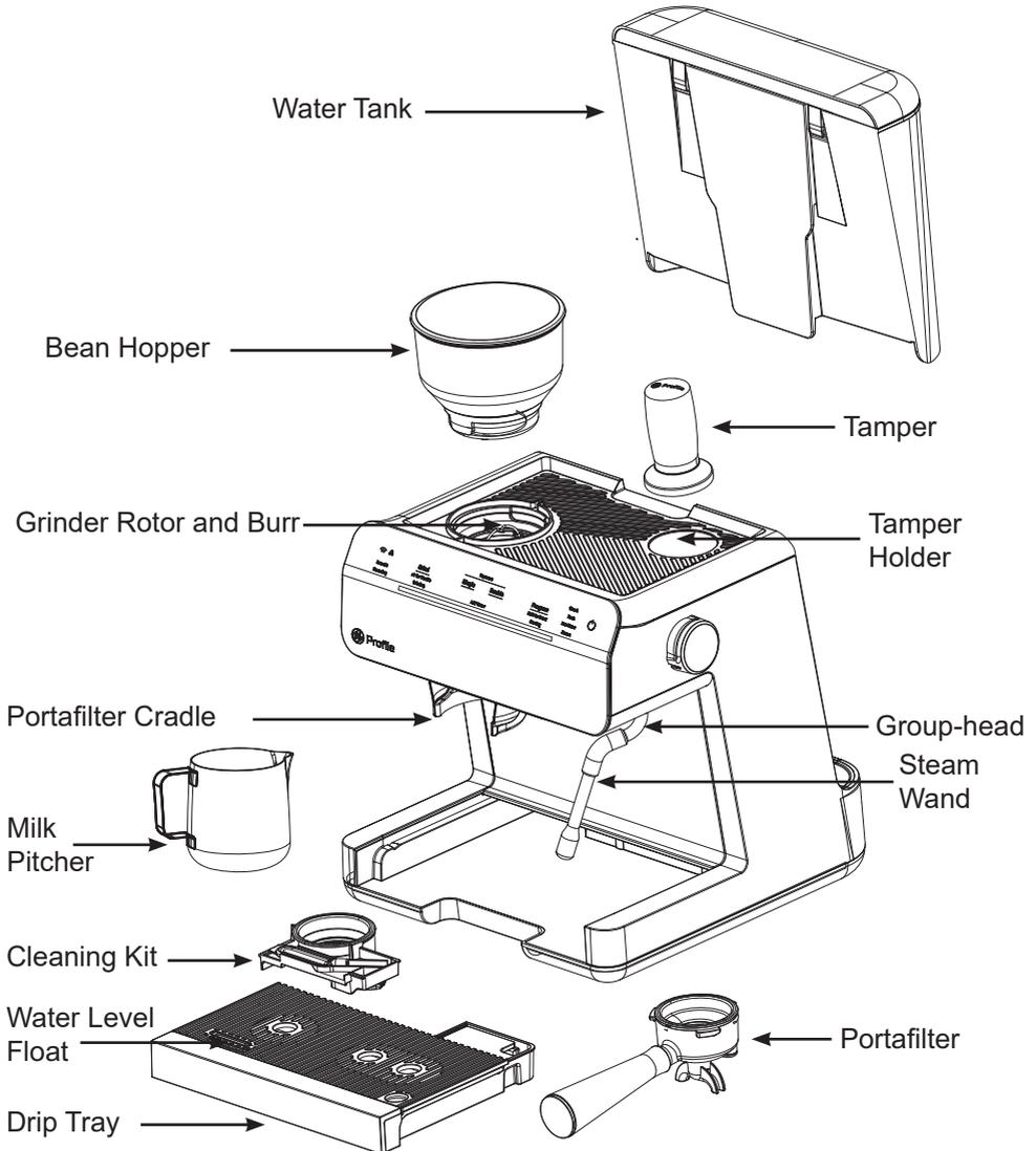
**NOTE:** When the water level float reaches the top of the drip tray, remove the tray and dispose of the liquid. Replace back in the machine before next use.
