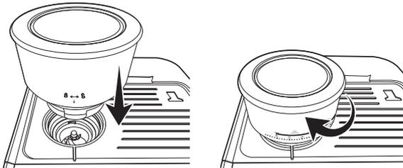
**NOTE:** The hopper grind size setting ranges from 0-15, 0 is the finest and 15 is the coarsest.
