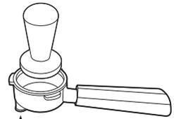
**NOTE:** Use the rubber pad on the bottom of the portafilter to level on the edge of a flat surface while tamping.
