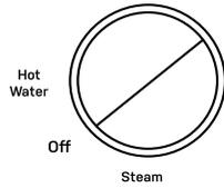
**NOTE:** Ensure knob is in the Off position when powering on the machine. Brew Function will not be available unless knob is in neutral position upon startup.
