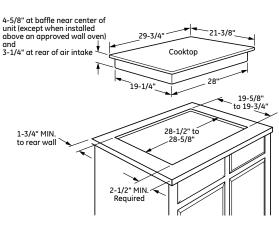
To insure accuracy, it is best to make a template when cutting the opening in the counter
