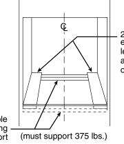
2 x 4 or equivalent runners level with bottom of cutout and flush with sides of cutout or solid bottom floor.
