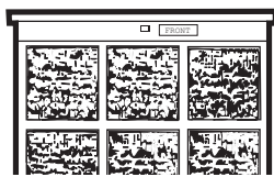
Dirty filter—Needs cleaning
