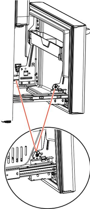
**A** Locate the height adjuster cam in the freezer door. Slightly loosen the three door attachment screws on both sides using a 3/8" hex socket driver.
