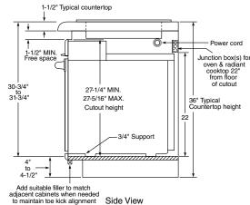
**Note**: For this installation, the bottom trim **will not** be flush with a typical 4" toe kick.
