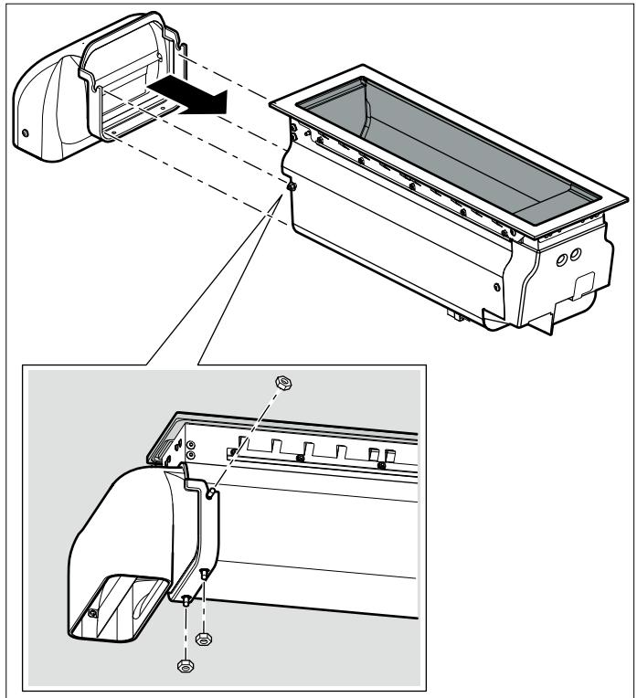
2. Insert the downdraft ventilation into the cut-out on the worktop.
