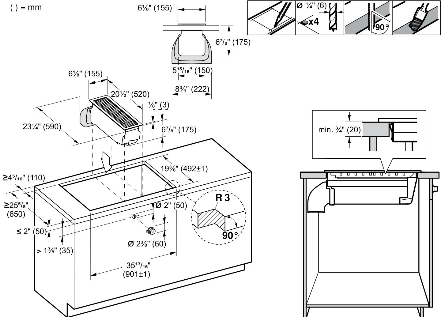
**Flush installation:** The appliance can be installed in the following temperature- and water-resistant countertops:
