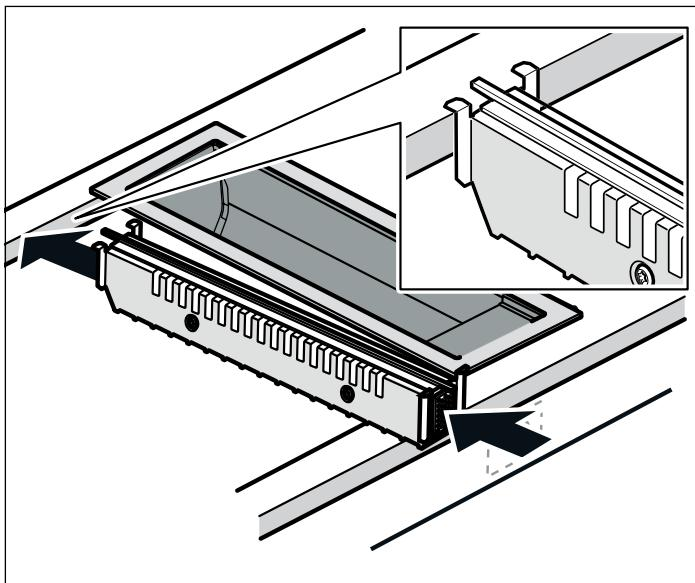
4. Press the connection strip firmly against the appliance; you should hear the appliance's clamp springs clicking into the recesses in the connection strip.
