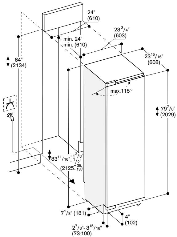
The door face dimensions are designed for a maximum gap of  $\frac{1}{8}$ " (3 mm).
