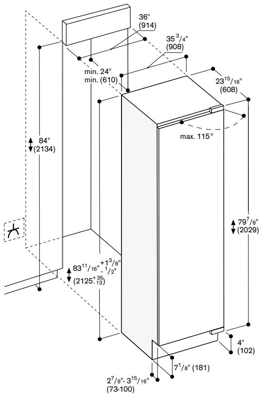
The door face dimensions are designed for a maximum gap of  $\frac{1}{8}$ " (3 mm).
