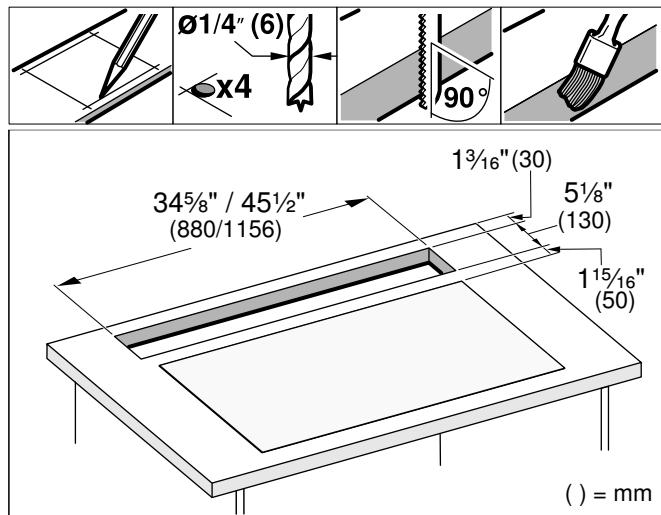
**Flush mounting:** Flush mounting into a countertop is possible.
