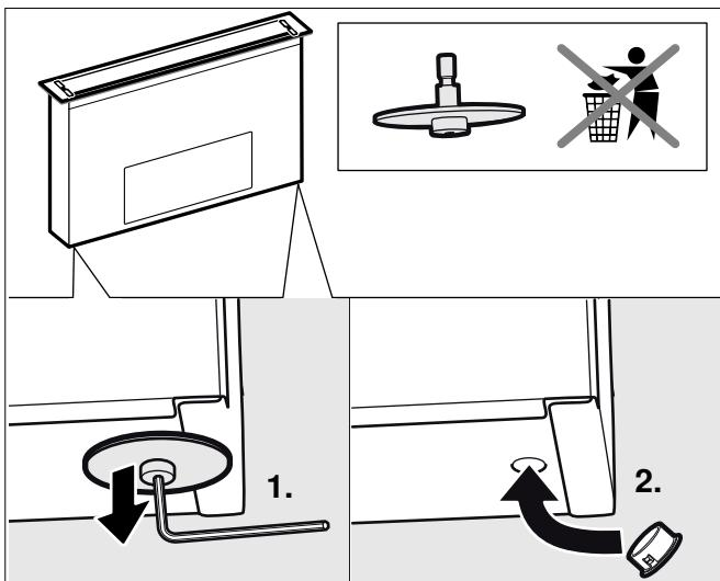
**Note:** Keep the transport locks. Re-mount transport locks before transporting the appliance (e.g. during a move).
