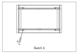
4. **Back Frame Installation:** Position back frame equal space top to bottom, side to side. Mark for 4 holes on the installed wood cleats, center punch and pre-drill with 1/16" drill bit. Secure frame with 4 Screws (E). See Sketch 7.
