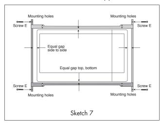
5. Install Air Deflectors top and bottom. Center (left and
