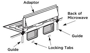
Push in securely until it is in the lower locking tabs. Take care to assure that the damper hinge is installed so that it is at the top and that the damper swings freely.
