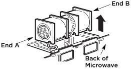
Roll the blower unit 90° so that fan blade openings are facing out the top of the microwave.
