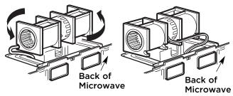
Gently remove the wires from the grooves. Reroute the wires through grooves on other side of the blower unit.
