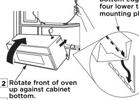
Insert a self-aligning screw through top center cabinet hole. Temporarily secure the oven by turning the screw at least two full turns after the threads have engaged. (It will be completely tightened later. Be sure to keep power cord tight. Be careful not to pinch the cord, especially when mounting flush to bottom of cabinet.
