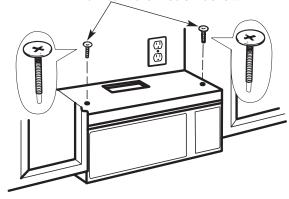
7 Tighten the outer two screws to the top of the microwave oven. (While tightening screws, hold the microwave oven in place against the wall and the top cabinet.)
