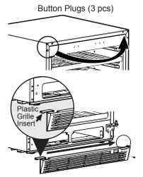
Transfer the plastic grille insert to the gap on the opposite side.
