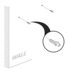
IMPORTANT: Consult an expert for the proper screws/bolts to use when attaching to various constructions. Screws provided do not attach to all wall construction types. Anchors are not required if brackets are installed in stud.
