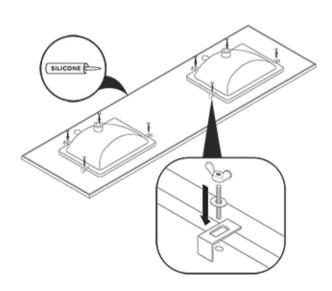
Apply silicone to the top of the cabinet (A) and place counter top with sink (B) already attached to It.
