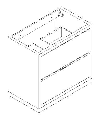
IMPORTANT: Consult an expert for the proper screws/bolts to use when attaching to various constructions. Screws provided do not attach to all wall construction types. Anchors are not required if brackets are installed in stud.
