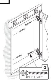
Level, then secure the medicine cabinet with the screws (**G**) through the mounting holes into the framing studs.
