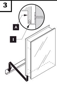
With assistance, rest the medicine cabinet on the bottom mounting bracket and hold it in place.
