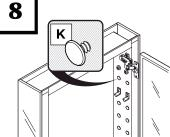
Fill remaining holes with the plugs (K).
