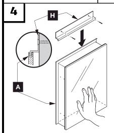
Hold the medicine cabinet (A) while it's placed on the bottom bracket, then secure by fitting the top bracket (H) on top of the medicine cabinet, and attach the top bracket (H) to the wall.
