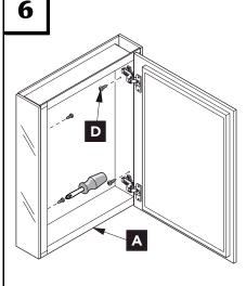
Attach mirrored side panels to the medicine cabinet using a screwdriver and provided screws (**D**).
