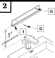
screws/bolts to use when attaching to various constructions.
