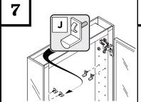
Push and twist the snapin pins (**J**) into place.
