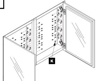
Fill the remaining holes with a plugs (K).
