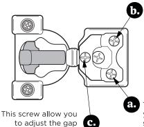
This screw releases cabinet's door and allows up and down adjustment.
