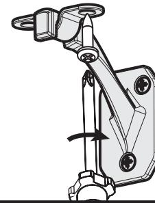
Drill 3/32 in. pilot holes and install the strap around underside of bracket arm.
