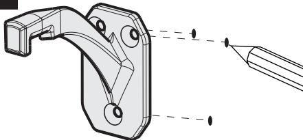
Position handrail bracket vertically in desired location and mark holes.
