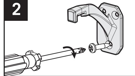
Drill 3/32 in. pilot holes and install bracket with 3 long screws.
