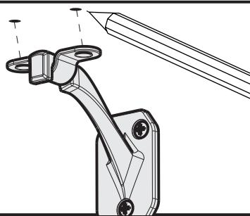
Position strap and mark holes on railing.
