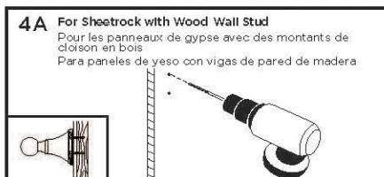
4A - Locate Studs before drilling.
