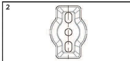
Position bracket on wall in desired location making sure that it is level.
