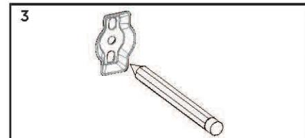
Mark (on the wall) locations of fasteners thru bracket using a pencil.
