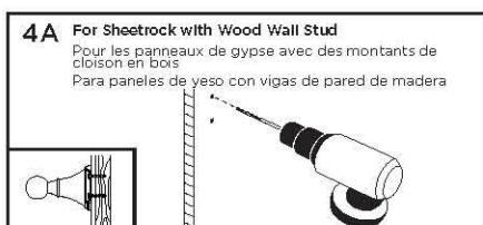
4A - Locate Studs before drilling.
