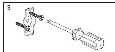
Attach brackets (confirm that clips face outward) to wall with fasteners provided and secure through drilled holes. Confirm that brackets are level.
