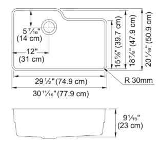
31-in. x 20-in. 18 Gauge Stainless Steel Undermount Single Bowl Workcenter Kitchen Sink. Create a highly efficient prep zone with the Orca 2.0 workcenter sink. The spacious bowl accommodates large cookware and big tasks. The integrated ledge system creates a multi-tiered bowl and allows accessories to work within the sink, creating a seamless workflow. ACCESSORIES INCLUDED: Bottom / Shelf Grid, Cutting Board, Roller Mat / Shelf Grid, Wire Basket, Strainer Basket and Drain Cover.
