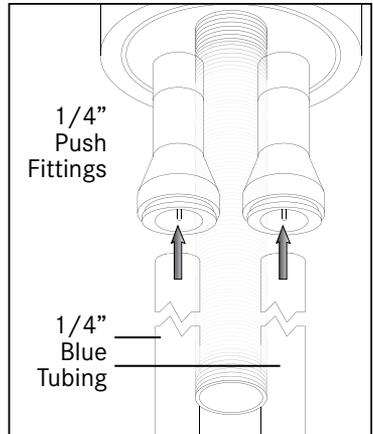
**6** Ensure proper hole is in place for the faucet. This faucet is designed for a 1-3/8" (35mm) mounting hole. Before inserting the faucet in the hole in the sink or counter top, make sure the O-ring is positioned in its seat and all hoses are secure. Place the faucet in the hole, orienting the spout towards the sink bowl.
