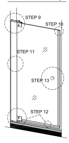
STEP 9 Set glass door into place by placing the pivot pin that sticks out of the bottom pivot plate into the hole in the bottom Pivot Bracket Arm. Slide top Pivot Bracket Arm down over the top pivot pin and tighten down the screws to secure it in place.
