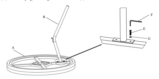
STEP 2 Attach the Leg Connector (C) to the Table Leg (B) using M6\*25 Screws (D) and Washers (G) then loosely tighten using the Allen Wrench (F).
