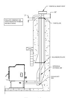
Figure 12 Venting through masonry chimney
