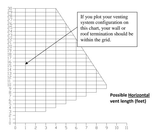
Let's imagine an installation consisting of a horizontal vent coming out at the back of the stove on a total distance of 8 feet. This horizontal run is followed by a Tee and a 6-foot vertical rise. This type installation is not acceptable. As you can see, the vent termination is clearly outside the allowed configuration zone on the chart. The venting system does not have at least one foot of vertical rise for each foot of horizontal run.
