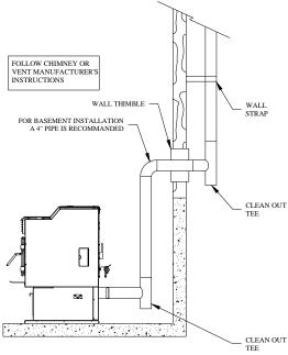
Figure 10 Basement installation
