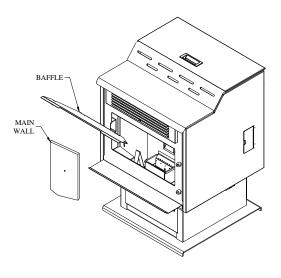
Figure 22 Baffle & exhaust access panel
