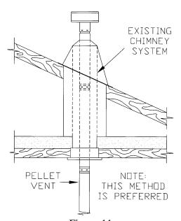
Figure 11 Venting through existing chimney
