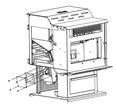
Figure 25 Exhaust blower cleaning
