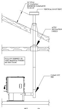
Figure 9 Venting through roof
