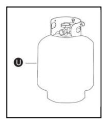
A dented, rusted or damaged propane cylinder may be hazardous and should be checked by your cylinder supplier. Never use a propane cylinder with a damaged valve connection.
