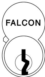
The "A" keyway is standard for I/C products and will be supplied unless otherwise specified. Falcon keyways shown here are equivalent to Best and Arrow I/C keyways of the same names.
