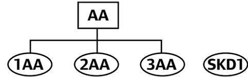
When all higher levels of master keys are to be disallowed, suffix **(NMK)** to the symbol of the key which is to operate. This means "not master keyed." Cylinder **1AA(NMK)** is operated by **1AA** only. The **AA** master is blocked from operation.
