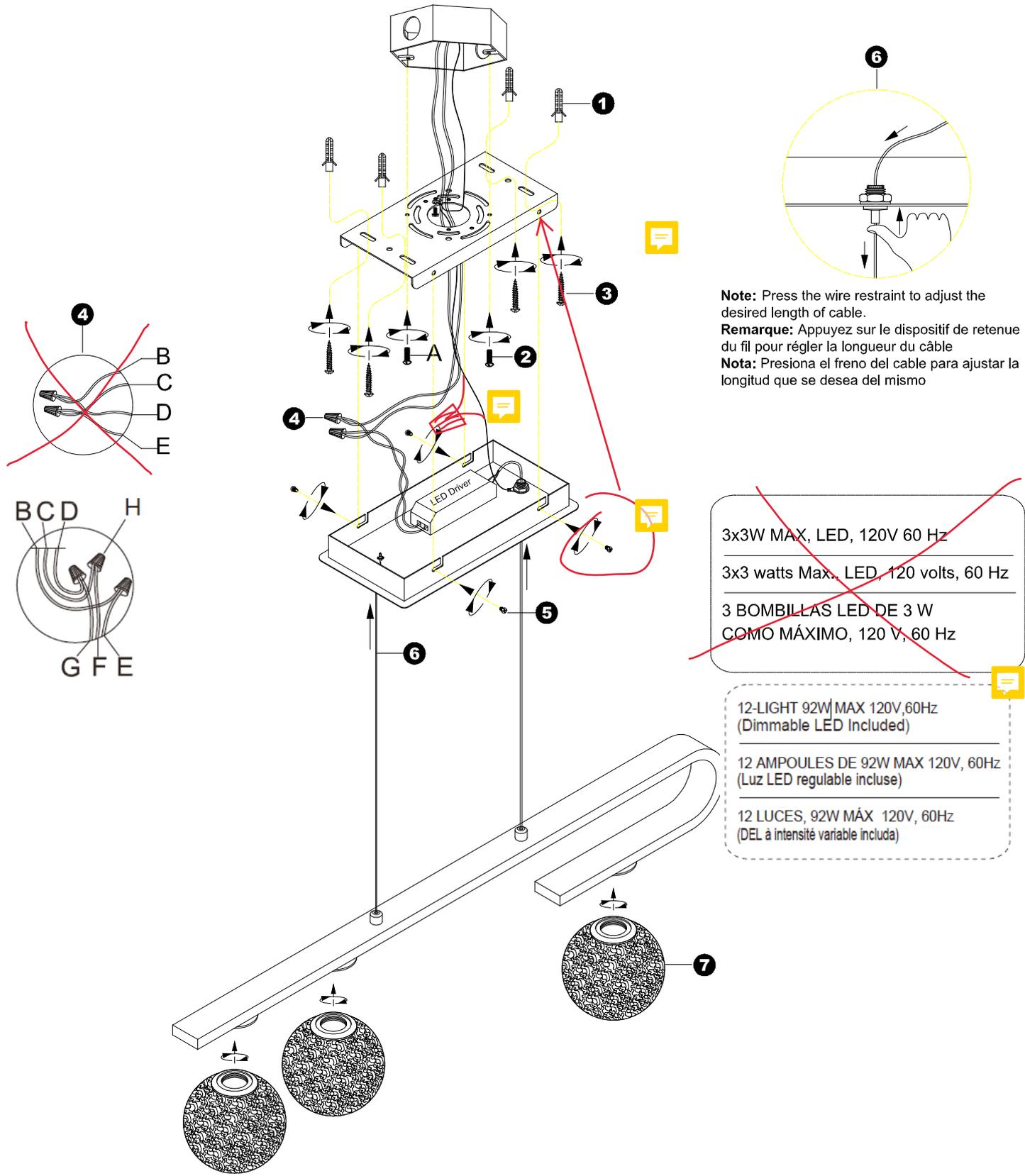
**Note:** Press the wire restraint to adjust the desired length of cable.
