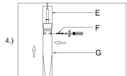
Step 4: Attach glass (G1&G2) using set screws (F).
