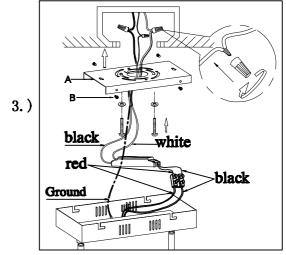
Step.3: Wire the fixture using the teminal block. The low voltage wires from the driver are already connected. Connect the black wire to the fixture's black wire and red wire to the fixture's red wire. Install the fixture to the mounting bracket using screws (B) provided.
