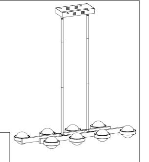
The fixture is designed to dim with a standard Triac forward phase dimmer. Dimming levels will vary by dimmer.
