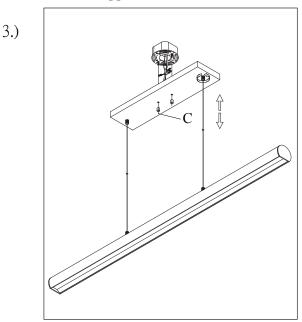
Step.3: Thread on the Decorative nuts(C) to the two studs until the fixture is secured to Mounting bracket(A).
