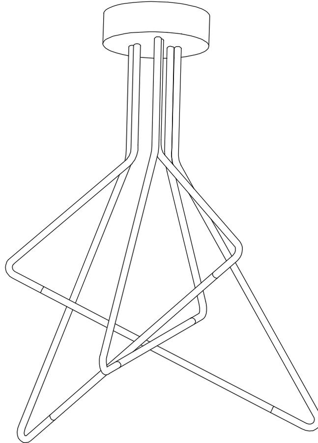
**WARNING: WIRES NEED TO BE CONNECTED TO DRIVER FOUND IN CANOPY AND SHOULD NOT CONECT DIRECTLY TO POWER SOURCE OR A SHORT MIGHT OCCUR.**
