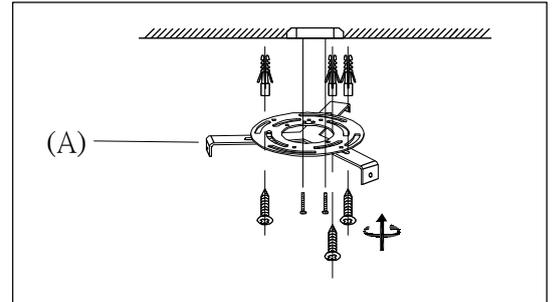
Step.1: Remove Bracket (A) from fixture and install to electrical box.
