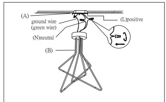
Step.2: Wire fixture to wires in outlet box.
