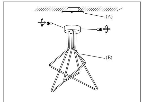
Step 3: Install Body (B) to Bracket (A) and tighten screws at the ends of the canopy to secure.
