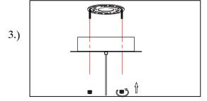
Step.3: Screw finials (C) onto mounting bracket (A) until canopy is flush with ceiling.
