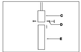
Step 4: Insert glass (E) into cup (C) and secure using screws (D) provided.
