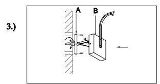
Step.3: Install fixture (B) to bracket (A) and tighten screws at the ends of the canopy to secure to wall.
